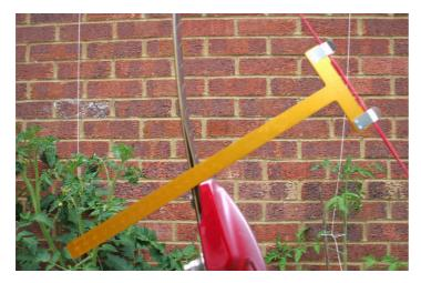
If the top limb measurement is greater than the bottom limb measurement this is referred to as a "Positive Tiller". If the top limb measurement is less than the bottom limb measurement this is referred to as a "Negative Tiller". Usually the difference between the two measurements is specified i.e. +5mm positive tiller means that the top limb measurement is 5mm greater than the bottom limb measurement. If the two measurements are the same this is called "Zero Tiller".
