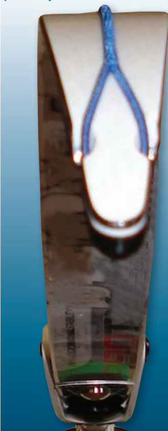
Limb tip off-centre requiring riser pocket adjustment
