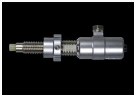
The pressure button is a spring mounted plunger against which the arrow shaft rests. During the bow power stroke the arrow shaft for a short time (around three thousandths of a second) pushes against the plunger which is depressed into the barrel (typically 1 – 2 mm ).
