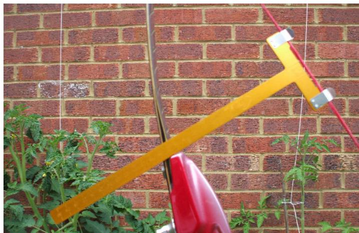
If the top limb measurement is greater than the bottom limb measurement this is referred to as a “Positive Tiller”. If the top limb measurement is less than the bottom limb measurement this is referred to as a “Negative Tiller”. Usually the difference between the two measurements is specified i.e. +5mm positive tiller means that the top limb measurement is 5mm greater than the bottom limb measurement. If the two measurements are the same this is called “Zero Tiller”.
